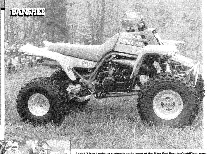
A trick 2-into-1 exhaust system is at the heart of the Moto Fast Banshee's ability to gene ate bottom-end power for woods plonking. Dico aluminum wheels with a combination: Fast Trekkers front and rear are Longwell's preferred wheel and tire choices for most woods events.
